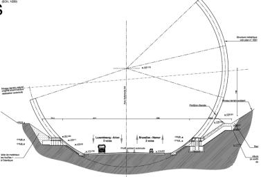
The structure is an arc and is modelled as a cantilever beam. The height is 60m and the radius is equal to 38.5m. The shape of the section is a square hollow section 2,25 m x 2,25m. The thickness is 40mm for lower third, 30 mm for the middle part and 20 mm for the upper third.
