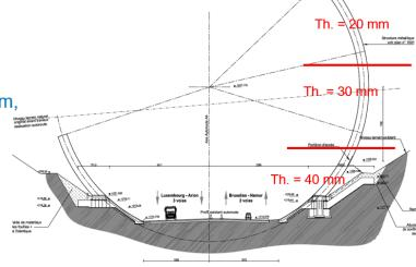
The structure is an arc and is modelled as a cantilever beam. The height is 60m and the radius is equal to 38.5 m. The shape of the section is a square hollow section 2,50 m x 2,5 m. The thickness is 40 mm for lower third, 30 mm for the middle part and 20 mm for the upper third.
