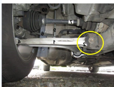
Lower control arm of a car
