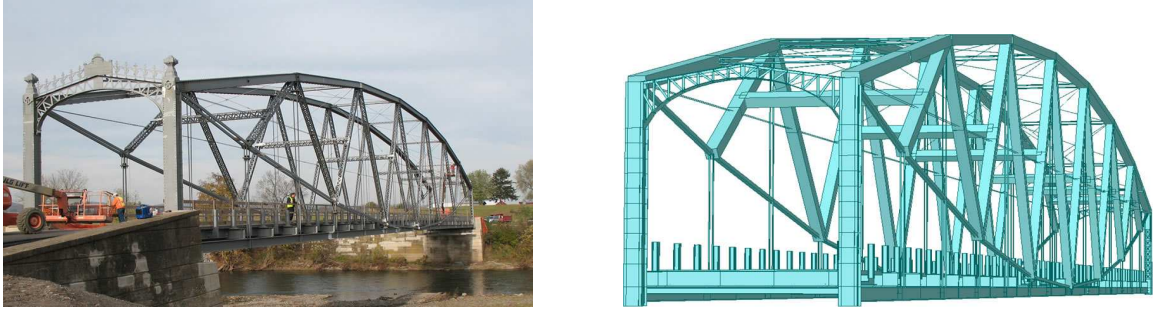
Figure 109: Finite element model of the Pine Creek bridge lenticular truss bridge ( http://fynitesolutions.com )
