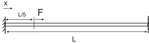
Figure 101: Fixed-fixed bar excited at L/5 in the horizontal direction
