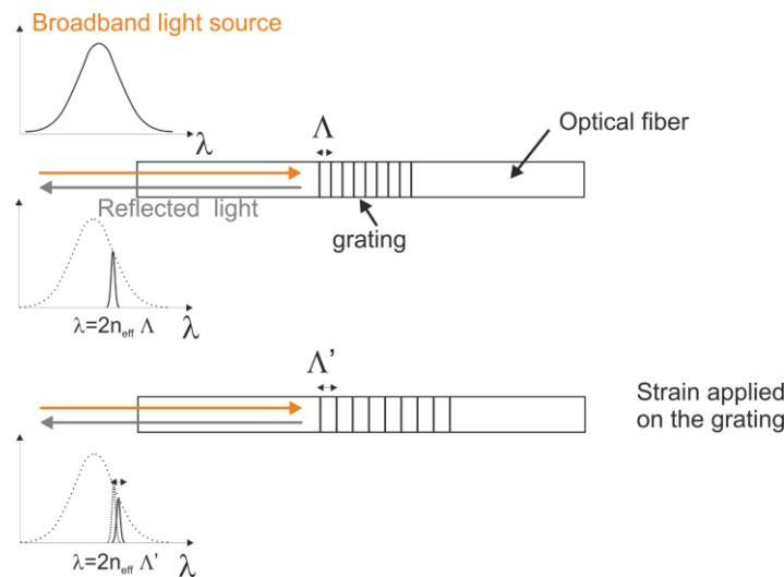
The change of reflected wavelength is proportionnal to the strain applied to the Bragg grating.
