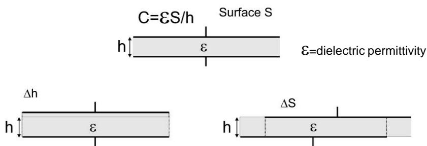
The change of capacitance is a measure of the relative displacement between the two electrodes
