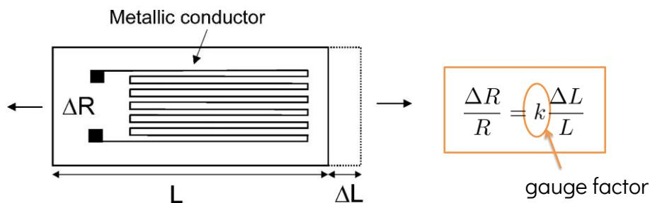
The change of resistance of the strain gauge is proportionnal to the **applied strain**
