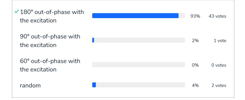
For an undamped 1DOF system, when excited with a harmonic force at a frequency corresponding to its natural frequency, the amplitude of the motion is
